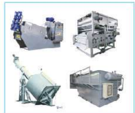
Screw Spress for Sludge Dewatering
